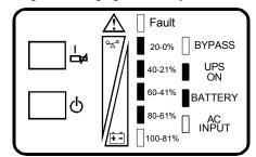
Figure 2 – Battery Mode Operation at 61-80% battery capacity
